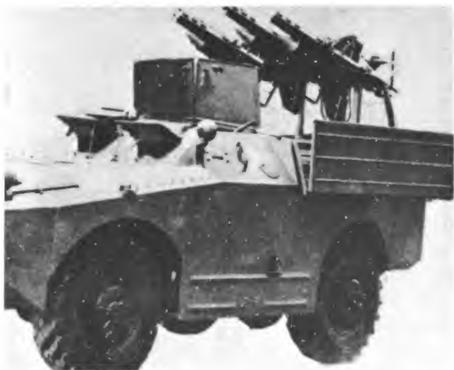
Figure 6-36. AT-1 SNAPPER. Shown here in a triple mount on a modified BRDM, this anti-tank wire-guided missile is probably being phased out in favor of the AT-3 SAGGER.
